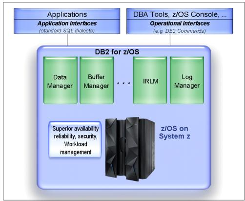
Figure 3. DB2 with no Accelerator attached
