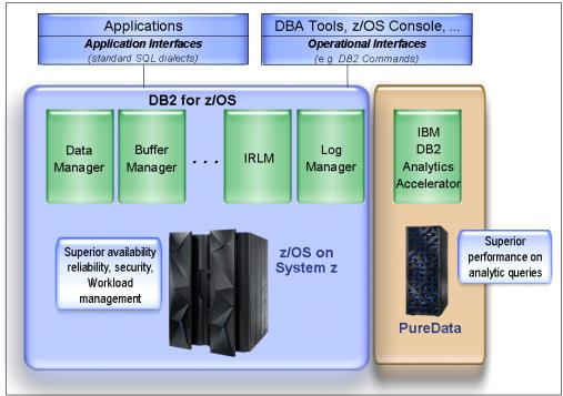
Figure 4. DB2 subsystem with attached DB2 Analytics Accelerator for z/OS
